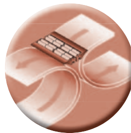
Head to tail transfer using two roller transfer assemblies positioned back-to-back
